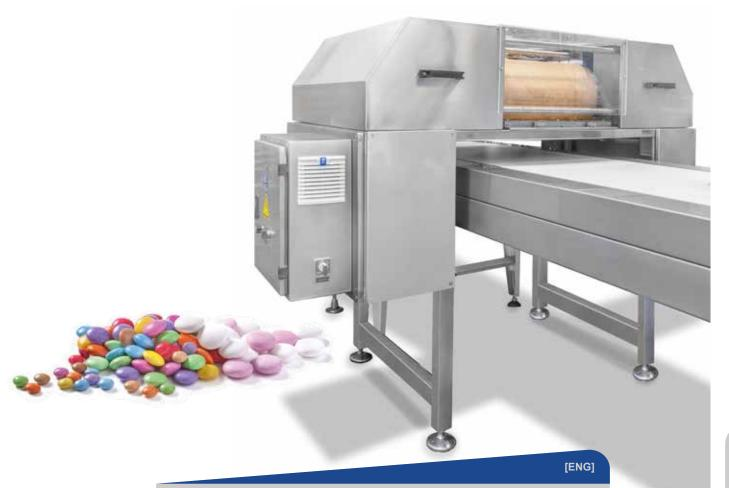
The chocolate lentil in-feeder is designed for small to medium capacity. With 60 to 150Kg/hour (depending upon lentil size), it is a versatile machine capable of producing all size of lentils, 0.9 to 20mm after coating. It is placed over a cooling tunnel, and can be used in conjunction with other machinery such as Drop depositor, enrober, C-Depositor or Vermicelli extruder, to produce a multi-functional plant.
